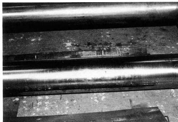
Fig. 8 Developed material (7%Cr high speed tool steels)
