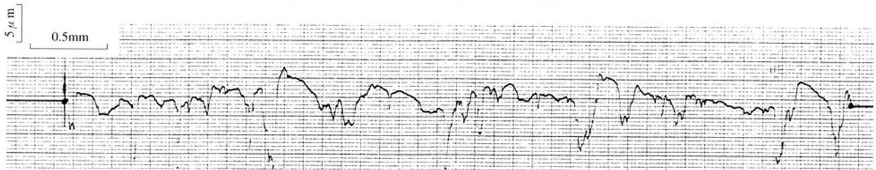
Fig.3 Roughness of roll surface after rolling (F3, 5069 ton) (Ra = 2.9  $\mu$ m, Rmax = 24.6  $\mu$ m)
