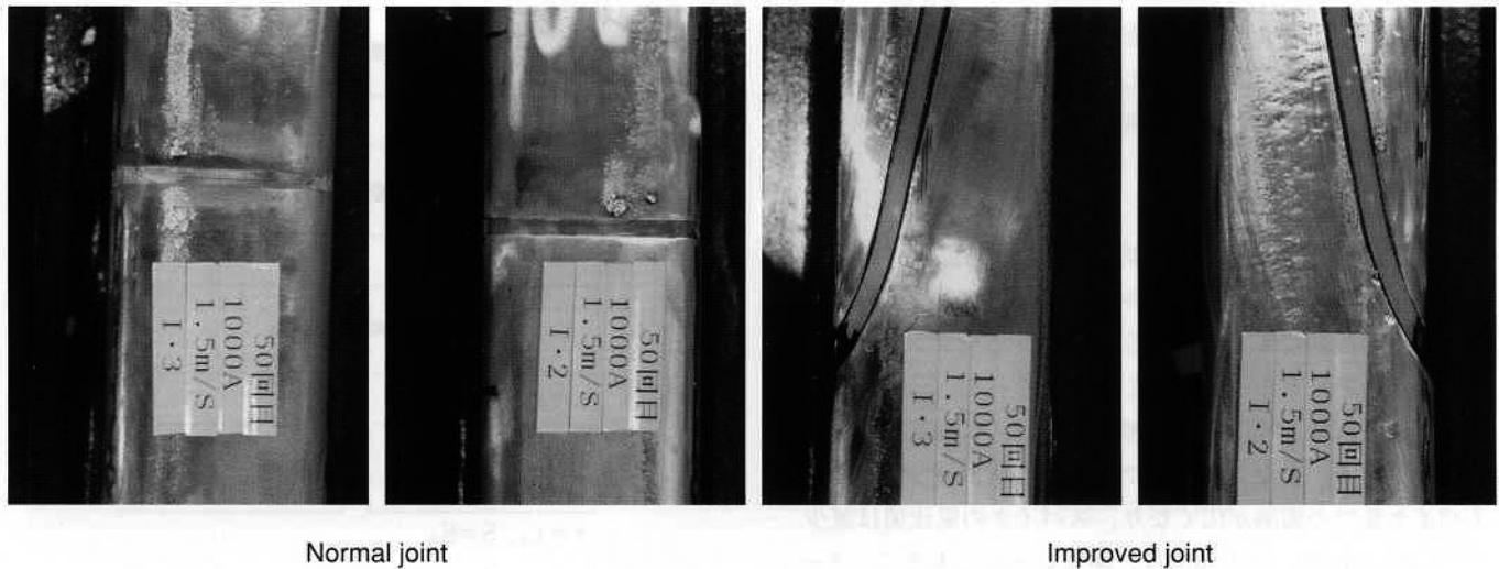
Fig.5 Arc-mark around the rails joint
