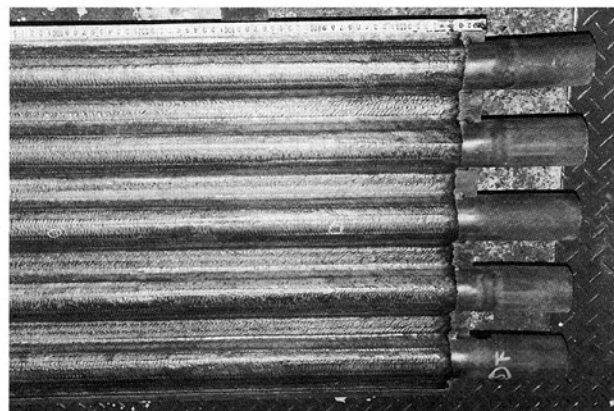
Fig.6 Part of weld water panel
