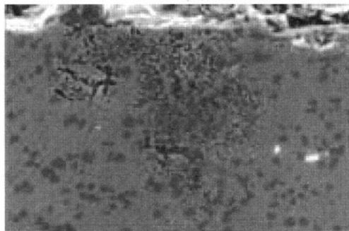
Fig.4 Microstructure of overlaying material after oxidation test
