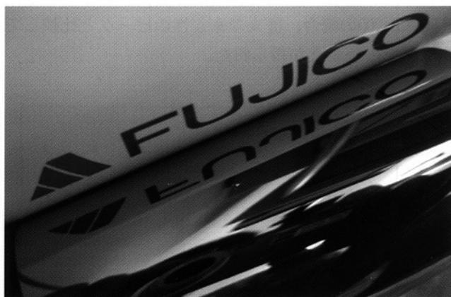
Fig.20 Appearance of specimen after mirror-like finishing
