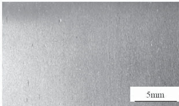
Fig. 12 Appearance of Fe-Cr alloy sheet after salt spray test for 1000 hrs
