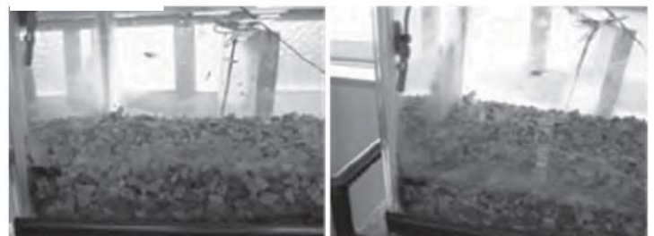
Fig.4 Water plant growth according to time elapsed of gravel without photocatalyst coating (up) and with one (down)
