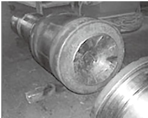
Fig.1 Appearance of the roll with a broken journal
