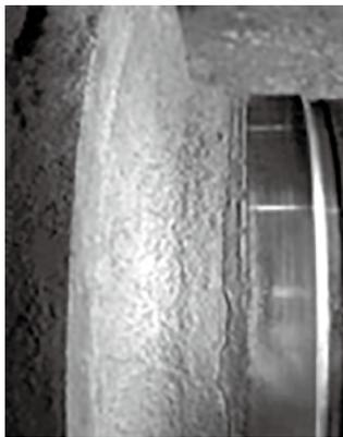
Fig.2 Appearance of the corroded journal
