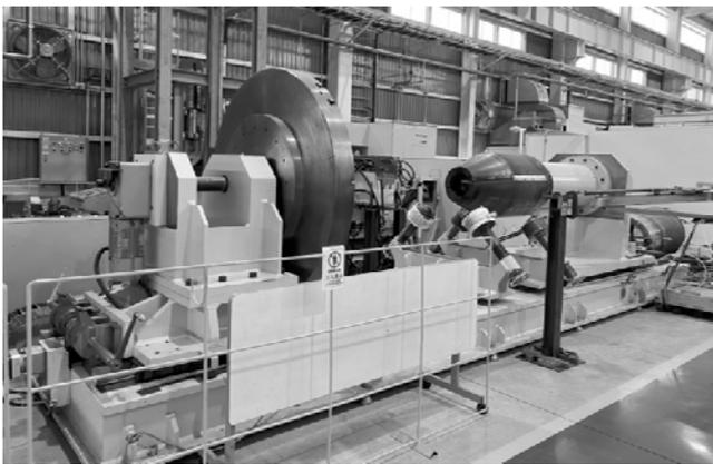
Fig.7 Expander for sleeve with large diameter
