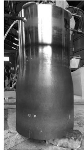
Fig.3 Expanded sleeve with small diameter
